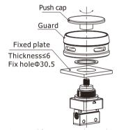
Disassembly: Remove the push cap, then remove the guard. Assembly: Install the guard, then to tighten the push cap.
