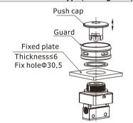
Disassembly: Untighten the guard first, then remove the push cap with the guard.
